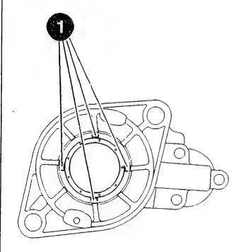
COMPONENT TESTING AND REPAIR Checking commutator end shield Check bushing for damage and scoring. Replace if necessary. Removal: Use puller (1) and spring collet to pull bushing out of commutator end shield. Puller: 0 986 617 243 Spring collet diameter 10 mm: 0 986 617 250
